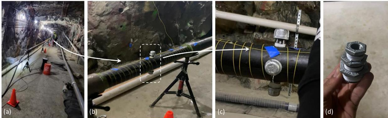
Figure 7. (a) A picture of the facility; (b) 1-m test section for leakage detection; (c) holes with caps on the 1-m test section; (d) reducers for hole size control
