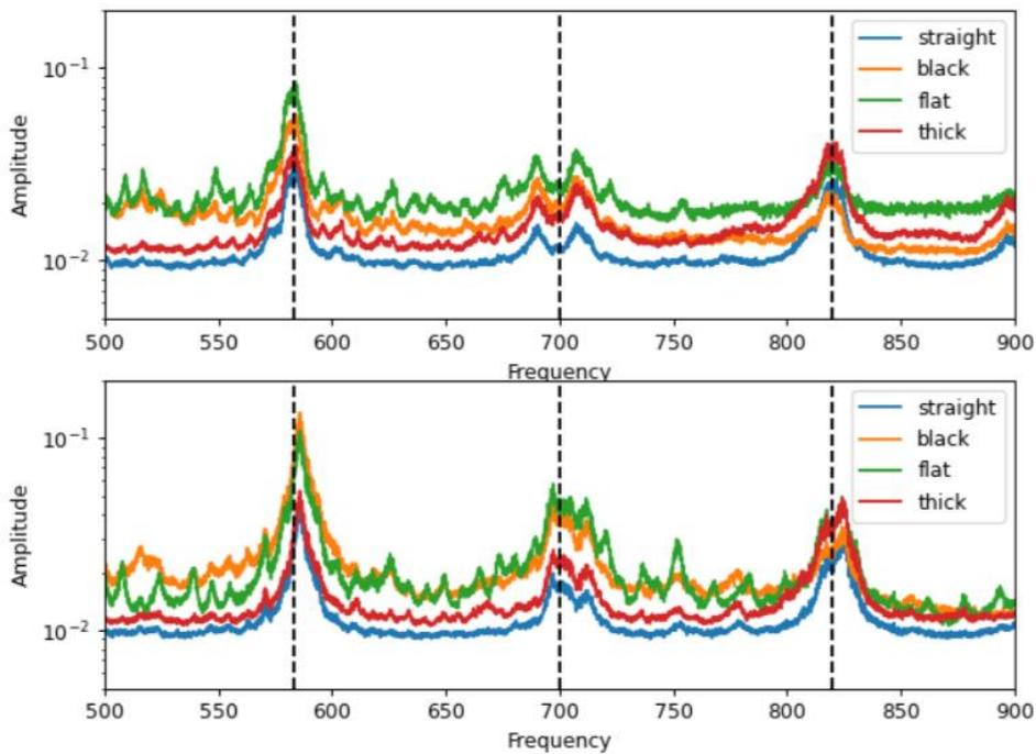
Figure 6. Averaged frequency spectrum of each fiber section, zoomed in between 500 Hz and 900 Hz. Top panel shows measurements with 5 supports, while the bottom panel shows those with 4 supports that simulates a scenario with a damaged support. Dashed line marked the estimated resonant frequency of three vibration modes.
