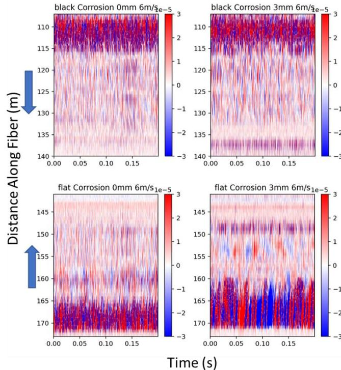
Figure 2. Examples of raw DAS data waveforms from black and flat fiber sections for Task#3. Left column shows the baseline without corrosion, and right column shows measurements with the pipe with 3-mm corroded depth. Blue arrow shows the gas flow direction in the fiber sections.
