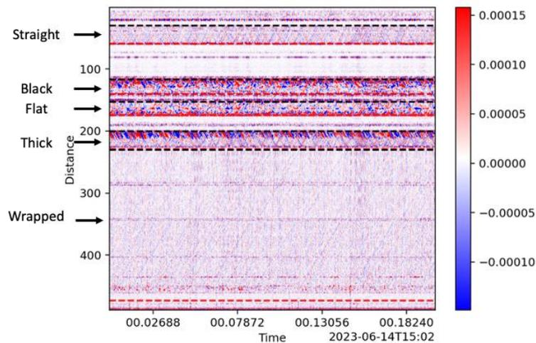
Figure 8. Raw DAS data recorded during the leakage experiment. The flow rate is 18 m/s, and with a 1' leakage point at the bottom. Black and red dashed lines are each fiber section's beginning and end points, prospectively.
