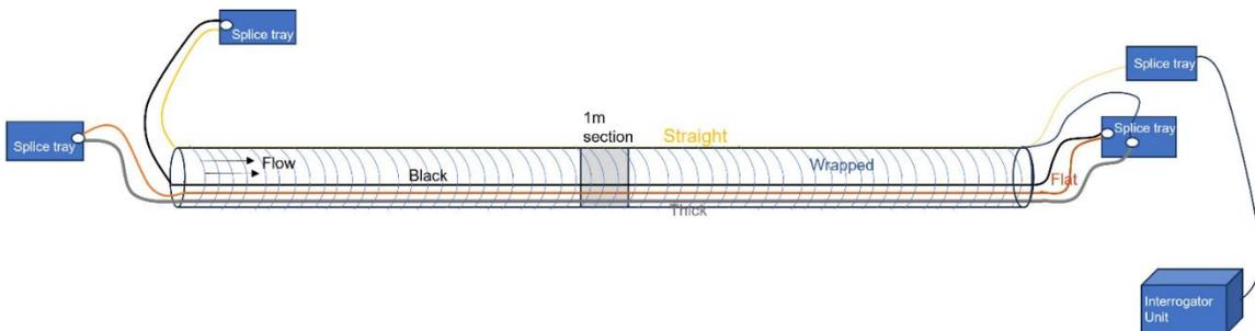
Figure 1. A schematic diagram showing the order of cable connection on the steel pipeline. The two black arrows indicate the direction of flow. Order of looped cable: Straight – Black – Flat – Thick – Wrapped.
