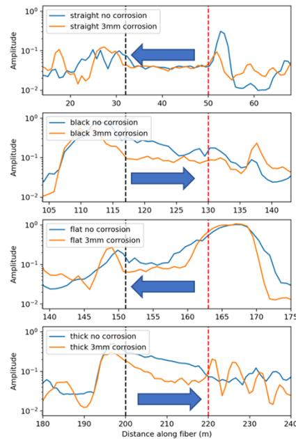
Figure 3. Vibration amplitude comparison at different fiber sections (straight, black, flat, and thick) between the corroded pipe and the baseline. These measurements were taken with a gas flow velocity of 6 m/s, and the data were filtered between 100 Hz and 1000 Hz. The arrow shows the flow direction compared to the fiber distance. Black and red dash lines mark the beginning and end of each section.
