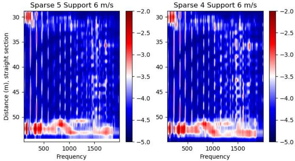
Figure 5. Frequency Spectrum of the straight fiber section with gas flow rate at 6 m/s. Vertical axis is the distance along the fiber/pipe, horizontal axis is frequency. Warmer color indicates higher amplitude at a certain frequency/location. The color is in log scale.
